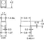
Note: A tolerance of ±0.1 mm applies to all dimensions unless otherwise specified.
