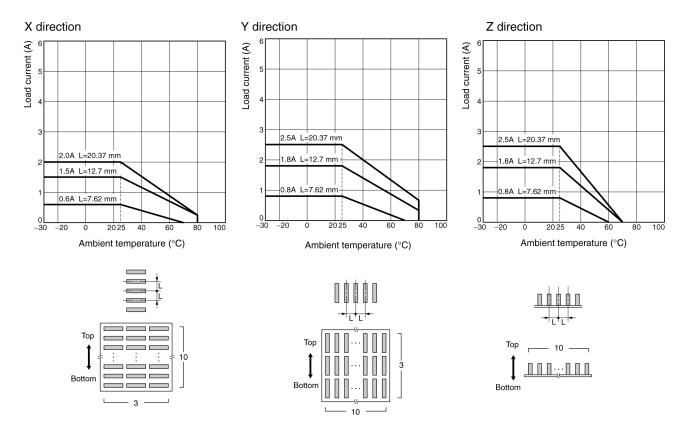
• Thirty Relays are soldered to the PCB at each given spacing.
