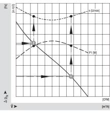
Air performance characteristics for forward curved centrifugal fans
