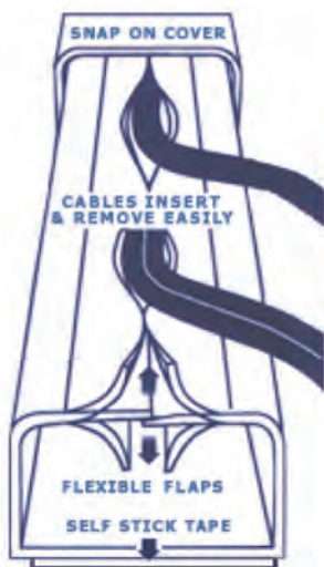
Wire Hider's Flexible Plastic Flaps Grips Wires during Installation.
