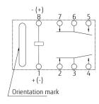
PC board mounting pad layout (TOP VIEW)
