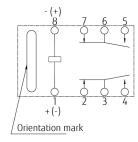
PC board mounting pad layout (TOP VIEW)
