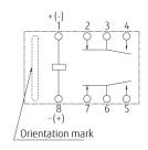
PC board mounting hole layout (BOTTOM VIEW)
