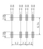
Note: Tolerance for PC board mounting hole/pad layout: +/-0.1.
