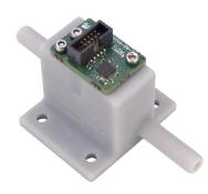
The FLS110 ports are sealed into the fixtures using O-rings. If you need to replace them, we recommend Nitrile 70 ShA, 1 mm inside diameter, 0.5 mm cross section.
