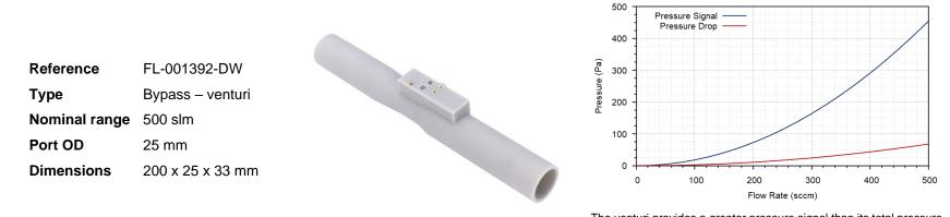
The venturi provides a greater pressure signal than its total pressure drop. The system pressure drop is shown in red.
