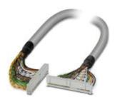
Round cable set; connection 1: IDC/FLK socket strip (1x 40-position); connection 2: IDC/FLK socket strip (1x 40-position); cable length: 4 m
