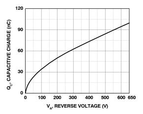
Figure 5. Capacitive Charge vs. Reverse Voltage
