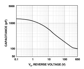
Figure 6. Capacitance vs. Reverse Voltage
