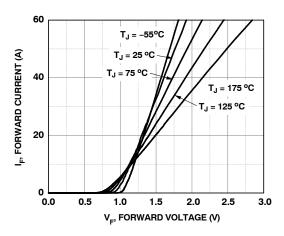
Figure 1. Forward Characteristics
