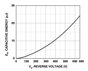
Figure 7. Capacitance Stored Energy
