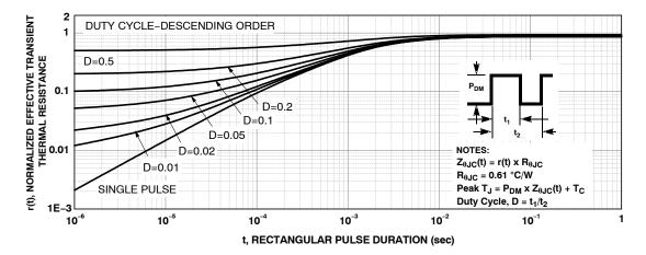
Figure 8. Junction-to-Case Transient Thermal Response Curve
