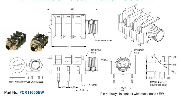
This 6.35mm Stereo jack socket has a metal nose and removable front earth washer. The body material is PBT UL V0 with an aluminium nose, and the contact material is brass / nickel plated. It has kinked PC legs for easy board assembly and is supplied with a washer and nut separate.
