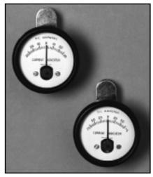
**Application:** This clip-on meter is designed to give a quick indication of current & direction of flow. There are no connections to be made, it simply clips over the conductor & operates on the induction principle.
