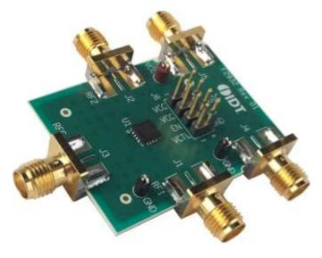
The F2932EVBI is a fully populated evaluation board which allows the customer to easily evaluate the F2932 RF switch.
