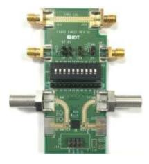
The F1977EVBI is a fully populated evaluation board which allows the customer to easily evaluate the device. Attenuation may be set using either the parallel control input or its serial control input (through external connection and control). A dip switch on the evaluation board allows one to set the attenuation state without off-board connections to the control inputs.
