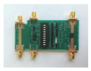
The F1956EVBI is a fully populated evaluation board which allows the customer to easily evaluate the F1956 digital step attenuator. Attenuation may be set using either the F1956's parallel control input or its serial control input. A dip switch on the evaluation board allows one to set the attenuation state without off-board connections to the control inputs.
