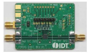
The F1951EVBI is a fully populated evaluation board which allows the customer to easily evaluate the F1951 digital step attenuator. Attenuation may be set using either the F1951's parallel control input or its serial control input. A dip switch on the evaluation board allows one to set the attenuation state without off-board connections to the control inputs.
