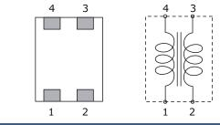
% The pin numbers shown here are for reference purposes only. Confirm the actual pin number arrangement with the exchanged specification documents.
