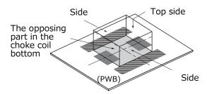
This power choke coil is different from the ferrite core-type that installs general concentration GAP. It has the leakage magnetic bunch distribution of the choke coil to the vertical direction. Please be cautious when using parts and circuit compositions which are easily affected by the leakage flux.
