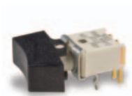
ET01J6ABE2 Horizontal Actuation SPDT
