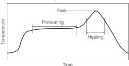
For soldering (Example: Sn/Pb)
