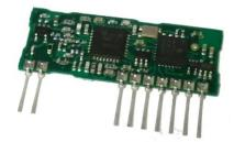
easyRadio Advanced (ERA) modules extend on the simplicity of previous easyRadio(02) modules by incorporating truly innovative features, including the ability to change bandwidth of the radio from 19.2KHz down to 12.5KHz, which means narrowband performance on a wide-band budget.
