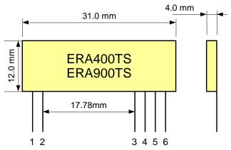
Pin Pitch 2.54mm PCB Hole Size 1.0mm
