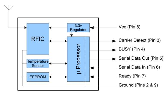
The Serial Data Input and Serial Data Output operate at the standard 19,200 Baud and the two handshake lines provide optional flow control to and from the host. The easyRadio Transceiver can accept and transmit up to 180 bytes of data, which it buffers internally before transmitting in an efficient over-air code format.
