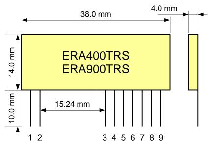
Pin Pitch 2.54mm PCB Hole Size 1.0mm
