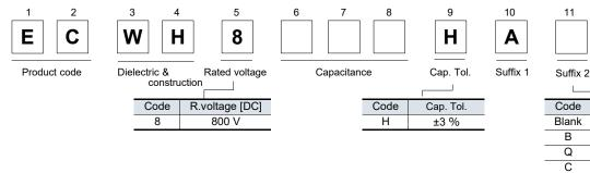
Rated voltage 800 V (Odd size taping)
