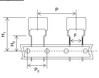
\*: H1 dimension is based on insertion machine "Panasert RH series" made by Panasonic. Consult with Panasonic technical staff when using other insertion machines.
