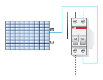
Wiring diagram for DC networks
