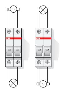
Wiring diagram for AC networks
