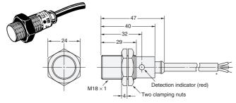
\* 6-dia. vinyl-insulated round cable with 3 conductors (Conductor cross section: 0.5 mm², Insulator diameter: 1.9 mm), Standard
