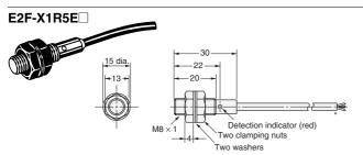
\* 3.5-dia. vinyl-insulated round cable with 3 conductors (Conductor cross section: 0.14 mm², Insulator diameter: 1 mm), Standard length: 2 m
