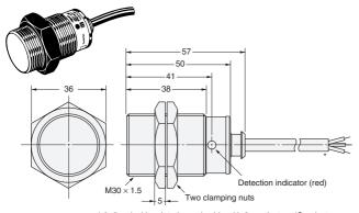
\* 6-dia. vinyl-insulated round cable with 3 conductors (Conductor cross section: 0.5 mm², Insulator diameter: 1.9 mm), Standard
