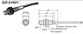
\* 3.5-dia. vinyl-insulated round cable with 2 conductors (Conductor cross section: 0.14 mm², Insulator diameter: 1 mm), Standard length: 2 m
