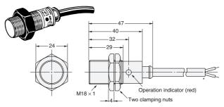
\* 6-dia. vinyl-insulated round cable with 2 conductors (Conductor cross section: 0.5 mm², Insulator diameter: 1.9 mm), Standard
