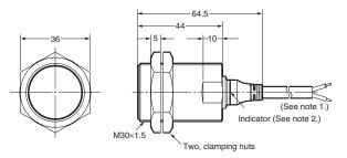
Note 1. 4-dia. vinyl-insulated round cable with 3 conductors (conductor cross section: 0.3 mm<sup>2</sup>; insulator diameter: 1.3 mm); standard length: 2 m 2. Operation indicator (yellow)
