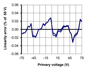
Figure 15: Typical linearity error at 25 °C
