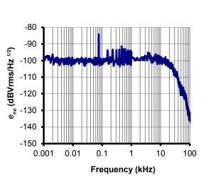
Figure 13: Typical noise voltage density of  $e_{_{\rm NO}}$  with  $R_{_{\rm M}}$  = 50  $\Omega$
