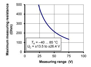
Figure 1: Maximum measuring resistance
