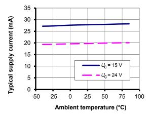
Figure 8: Supply current function of temperature
