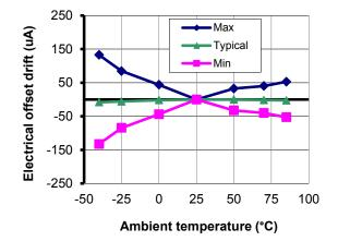
Figure 3: Electrical offset thermal drift
