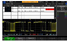
Figure 17. CAN-FD decode and trigger.
