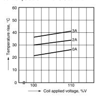
4-(3). Coil temperature rise (2 Form C 2 coil latching type) Tested sample: DS2E-ML2-DC12V Point measured: Inside the coil
