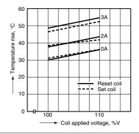
4-(4). Coil temperature rise (4 Form C 2 coil latching type) Tested sample: DS4E-ML2-DC12V Point measured: Inside the coil Ambient temperature: 20°C 68°F
