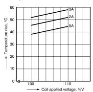
4-(2). Coil tempeature rise (4 Form C single side stable type) Tested sample: DS4E-M-DC12V Point measured: Inside the coil
