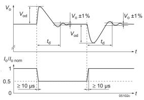
Fig. 12 Typical dynamic load regulation of output voltage
