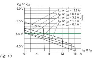
5 V tracking output  $V_{o4}$  versus  $I_{o4}$  (powertrain 1) or  $V_{o3}$  versus  $I_{o3}$  (powertrain 2).  $V_i = V_{i \text{ nom}}$
