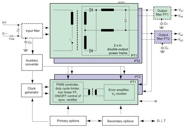
Fig. 7 Block diagram. Powertrains PT1 and PT2 have isolated outputs. Pin allocation see table 13
