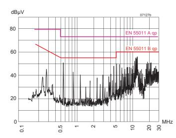
Fig. 21b CP 1001-7RB1 Typ. conducted disturbance voltage at the input ( $V_{i nom}$ ,  $I_{i nom}$ , resitive load, quasi peak).
