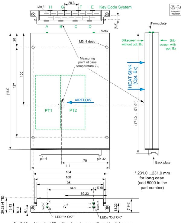
$\bigcirc$  =  $\oslash$  4.5 Alternative LED positions for customer-specific models with long case: a = "In OK", b = "Out 1 OK", c = "Out 2 OK" (front panel XMD168-G)
