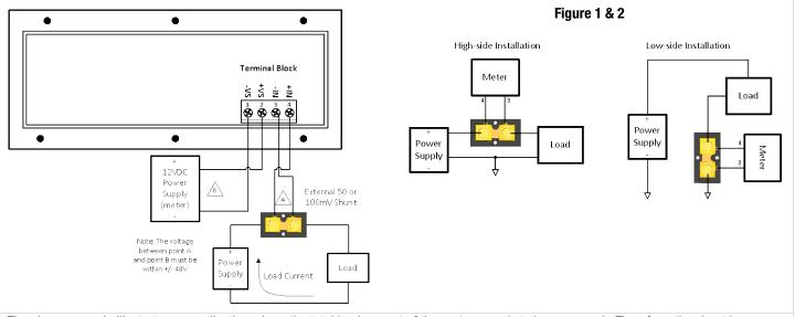
The above example illustrates an application where the total load current of the system needs to be measured. Therefore, the shunt is connected in series with the system load, at the same time, the shunt measurement points connected to terminals 3 & 4, as shown. The potential difference (VDC) across these points is converted and displayed as DC current, and indicates total system load. This is a high-side installation. See Figure 1 & 2 above for and example of low-side installation.
