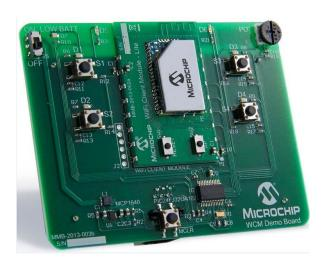
The Microchip WiFi Client Module Development Kit 1 is designed to enable the user to quickly and easily connect to a cloud based server such as Amazon AWS. The kit includes the WCM demo board utilizing a Microchip WiFi Module MRF24WG0MA and an application microcontroller PIC32. The device allows commissioning to router and then connects to an Amazon AWS server. The AWS account and AMI must be established prior to module commissioning. Microchip offers a free AMI image on Amazon AWS.
