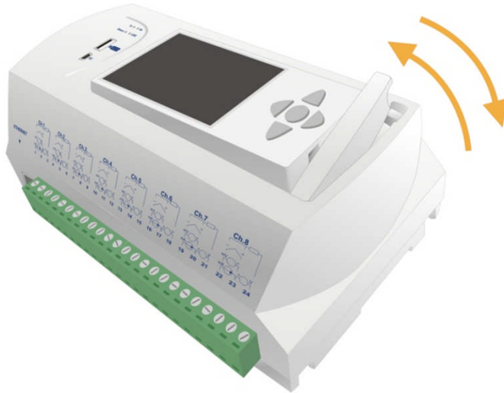
Fig. 10 – Attaching and detaching the Data Logger DISPLAY
