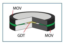
Using proprietary computer-aided design techniques to model performance, Bourns engineers created the equivalent function of a discrete MOV and GDT in series. After assembly of the core, leads are attached, and the unit is epoxy coated. The result is a familiar radial disc MOV package that is only slightly thicker and of substantially smaller diameter than similarly rated conventional devices.
