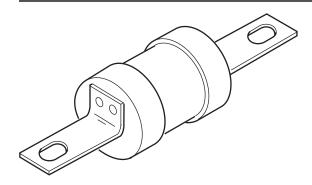
CATALOG SYMBOL: DD INDUSTRIAL HRC FUSE CENTER BOLTED TAGS PACKAGE QUANTITY: 5 80KA INTERRUPTING RATING MOUNTS IN 200DF FUSEBLOCK
