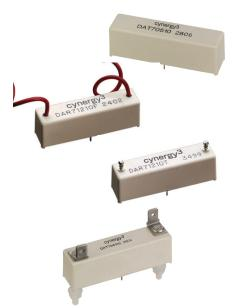
Very high isolation voltages, up to 15kV, are achieved through the use of high vacuum reed switches with either Rhodium or Tungsten contacts and make these relays suitable for high reliability applications, such as cardiac defibrillators, test equipment and high voltage power supplies.
