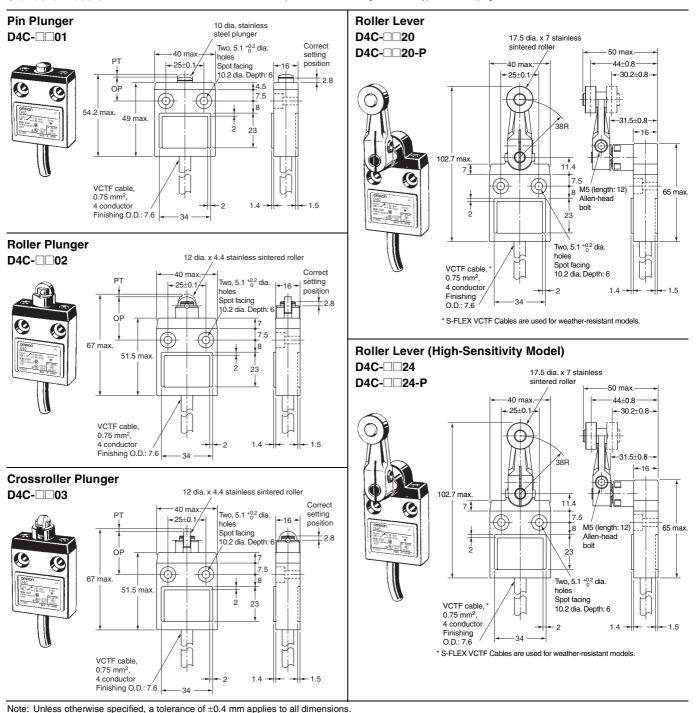
Model D4C-020 D4C-024 Operating D4C-001 D4C-002 D4C-003 D4C-020-P D4C-024-P characteristics Operating force OF max. 11.77 N 11.77 N 11.77 N 5.69 N 5.69 N Release force RF min. 4.41 N 4.41 N 4.41 N 1.47 N 1.47 N Pretravel PT max. 1.8 mm 1.8 mm 1.8 mm 25° 10°±3° Overtravel OT min. 3 mm 3 mm 3 mm 40° 50° Movement Differential MD max. 0.2 mm 0.2 mm 0.2 mm 3° 3° 28.5±1 mm 28.5±1 mm Operating Position OP 15.7±1 mm --------
