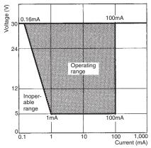
However, even when using microload models within the operating range shown above, if inrush current or inductive voltage spikes occur when the contact is opened or closed, then contact wear may increase and so decrease the service life. Therefore, insert a contact protection circuit where necessary.
