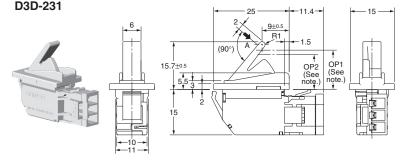
Note: The dimensions OP1 and OP2 apply to the D3D-211 only. The D3D-221 and D3D-231 are SPST-NC and SPST-NO respectively and so therefore have only one corresponding dimension here (OP).
