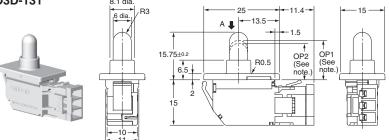
Note: The dimensions OP1 and OP2 apply to the D3D-111 only. The D3D-121 and D3D-131 are SPST-NC and SPST-NO respectively and so therefore have only one corresponding dimension here (OP).
