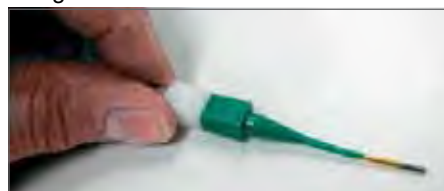
Plastic tool with contact in proper position.
