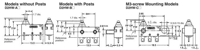
Mounting Hole Dimensions (Reference) Mounting Hole Dimensions (Reference)
