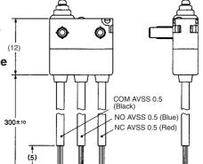
**Molded Lead Wires on Left-side**
