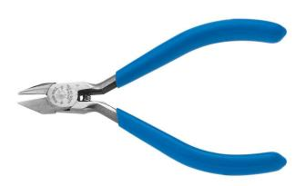
Narrow jaw and hinge for delicate work in tight areas. Sharp pointed nose for precise tip cutting. Spring-loaded action for self-opening. Short jaws and beveled cutting edges permit close cutting of wire. Induction-hardened cutting knives for long life. Hot-riveted joint ensures smooth action and no handle wobble. Plastic-dipped handles for comfort and ease of identification. Custom, US-made tool steel.
