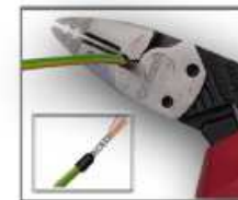
Aderendhülsen crümpen Crimping of ferrules 1,5 - 2,5mm 2
