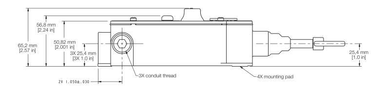
Figure 5. 2CPS Dimensional Drawing
