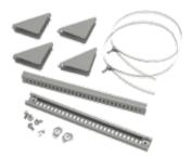
Use to mount CONCEPT, Networking and wall-mount enclosures to poles of various sizes and shapes. Simply attach the plated steel channel bar to the mounting holes at the back of the enclosure and wrap the stainless steel strap around the pole and through the bar. Kit includes two mounting channels, two straps suitable for 3-in. (76-mm) to 12-in. (305-mm) diameter pole and mounting hardware.
