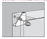
Panel Conversion Kit adapts enclosure for mounting standard NEMA-style panels in CONCEPT enclosures. Bracket attaches to rear collar stud. Kit includes four adapter plates and hardware for mounting panel.
