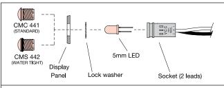
LED 5mm bi-lead trim lead length .250" ± .01" (5.58mm) .032" to .125", Panel Hole: .312" (8.0mm) Panel Thickness
