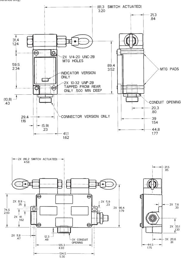
Momentary Cable Pull Limit Switches: For Signaling Applications
