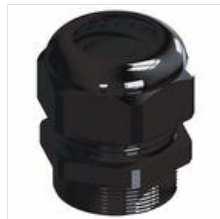
Cable Glands, Straight, Black, Nylon, PG13.5, 20.7 mm Hole Dia., 6.0 mm - 12.0 mm Cable, 9.0 mm Thread Length
