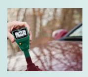
Extech's CG304 offers a non-destructive way of measuring the thickness of ferrous and non-ferrous substrates with auto recognition of the material being measured. Unique Bluetooth® interface feature wirelessly transmits measurement data to your PC for further analysis and to generate a documented report.
