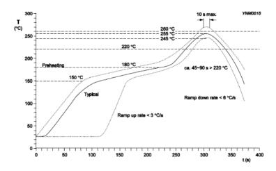
Solid line: Typical process (terminal temperature)
