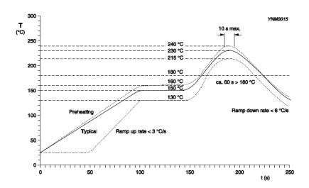
Solid line: Typical process (terminal temperature)
