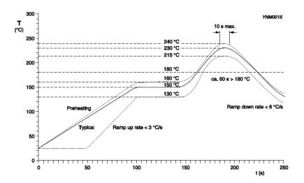
Solid line: Typical process (terminal temperature)
