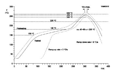
Solid line: Typical process (terminal temperature)
