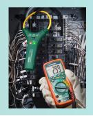
Expand your meter's capabilities to measure AC Current up to 3000A. Fit most MultiMeters or Clamp Meters with standard shrouded banana plug sockets. Flexible clamp jaw easily wraps around bus bars and cable bundles where standard clamp adaptors and meters can't. The thin 7.5mm cable diameter easily fits into tight spaces. Choose between a 10" (25.4cm) or 18" (45.7cm) clamp cable length.
